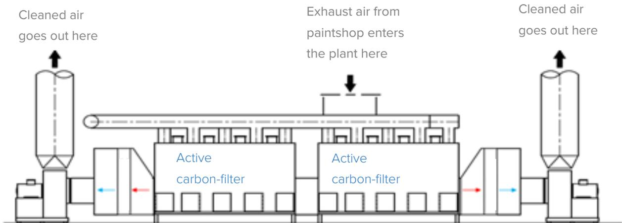
The plant is 20 meters in length, 10 meters in width, and 5 meters in height.
